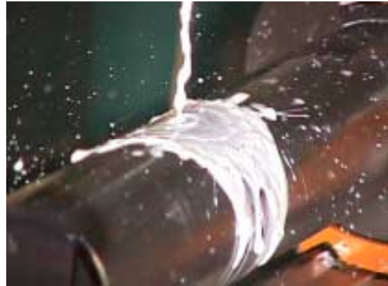
Figure 1. Cutting Fluid Jet Impinging on a Rotating Workpiece
